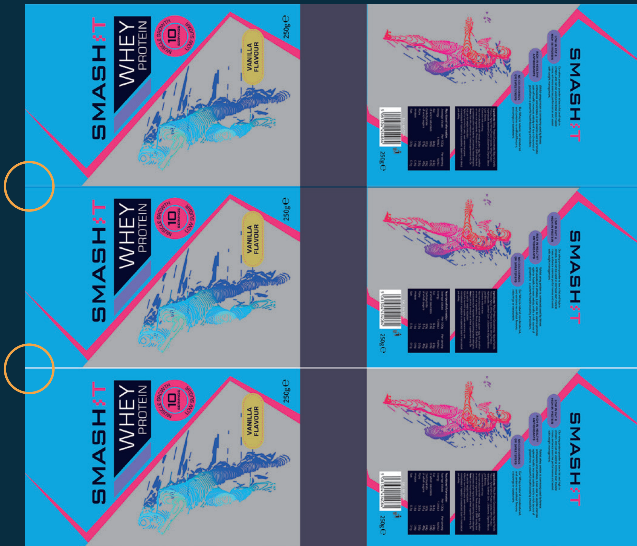
Possible overlap or gap within the repeat printing process.
